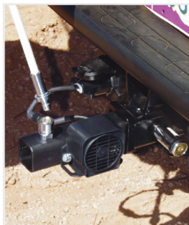
HM-QDA (shown) Powered, Quick Connect Whip Mount with 107dB Backup Alarm
